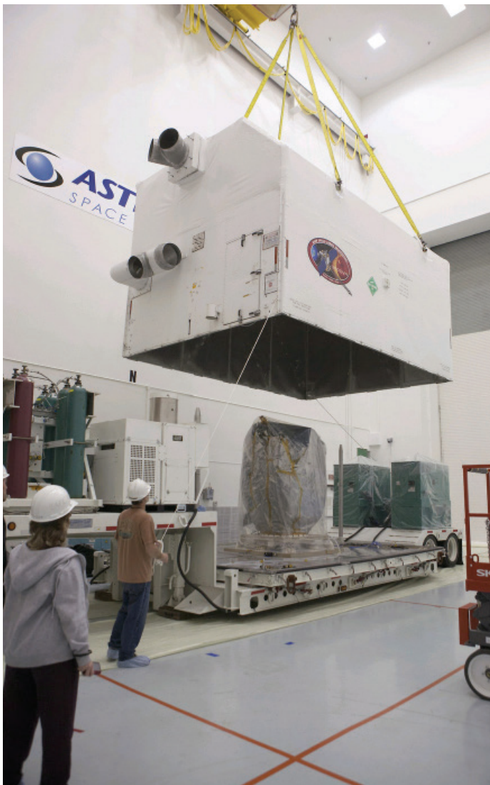
NOAA's Deep Space Climate Observatory spacecraft, or DSCOVR is being unwrapped for the New Year and prepared for launch. In this photo, DSCOVR, wrapped in plastic, comes into view as the protective shipping container is lifted from around the spacecraft at the Astrotech payload processing facility in Titusville, Florida, near NASA's Kennedy Space Center. Photo credit: NASA
